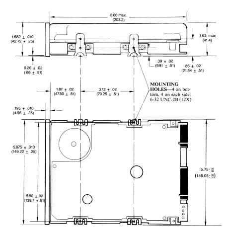
Dimensions are in inches (mm). NOTE: Mounting screws must not extend more than .25 inch inside the drive.
