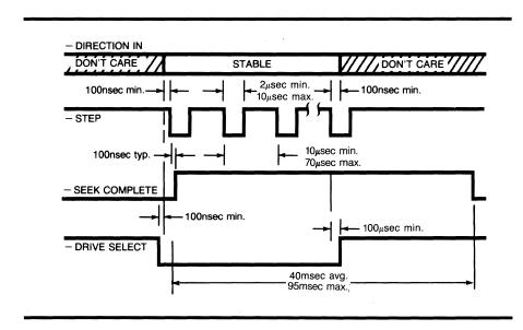
FIGURE 12: Buffered-Seek Timing
