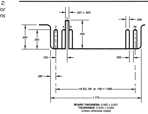
FIGURE 2: J1 Connector Dimensions
