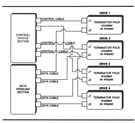
FIGURE 9: Radial Configuration
