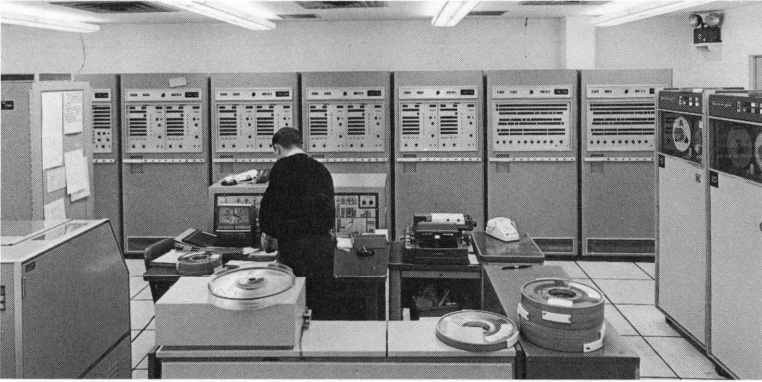
The BUIC III development computer at SDC—a duplicate of an operational military computer, the Burroughs AN/GSA-51. BUIC was designed to conduct air defense if SAGE became inoperative.
