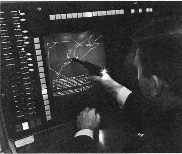
(Left) SDC integrated a computer-aided instruction system into the operational BUIC air defense consoles. This student is using light-pen in response to the lesson frame on the scope.
