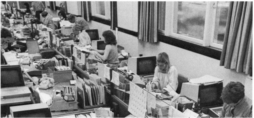
SDC's TEXT II electronic publishing system in use. Newspaper advertising department employees keyboard the copy for display and classified ads; the TEXT II system performs automated composition, pricing, and billing.
