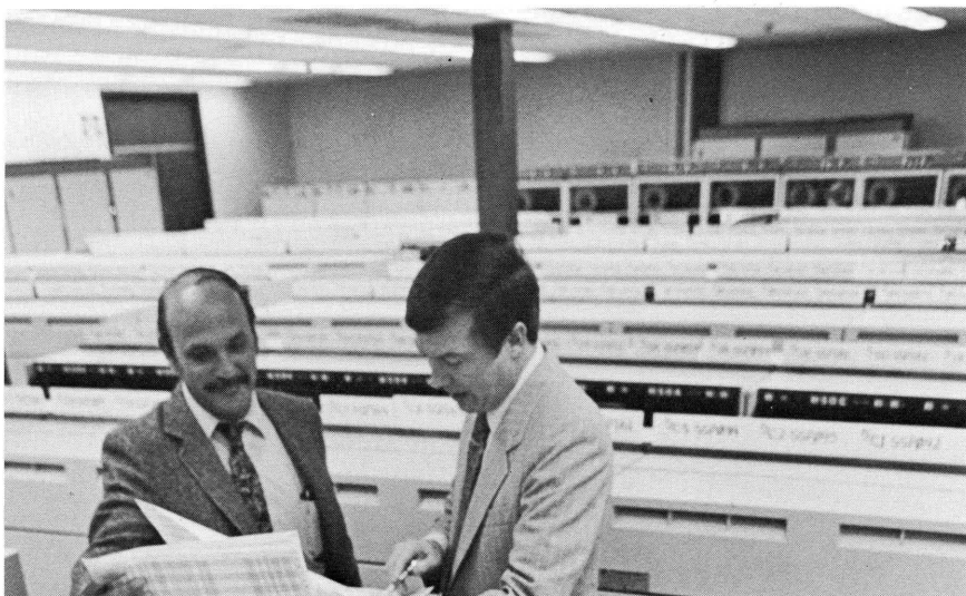
Of the rows of disk drives attached to SDC's Amdahl 470 V/7 computer, sixty are dedicated to on-line storage of SDC Search Service data bases. Project manager Thomas F. Collins ( right ) reviews requirements for 80 billion characters of storage with Richard I. Springer.
