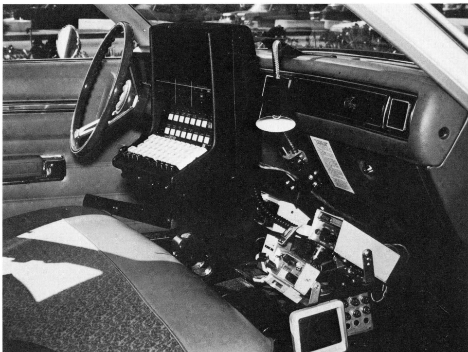
A Los Angeles Police Department patrol car equipped with components of SDC's ECCCS system is a major attraction of a November 1978 Open House. The interior of the car ( bottom photo ) shows one of the 850 ECCCS terminals used by officers for digital communication with a central computer, alleviating overcrowded voice channels.
