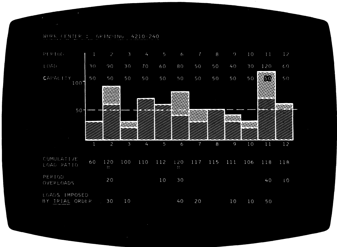
Figure 37. Example of how a system can display overloads caused by an order accepted within normal lead time
