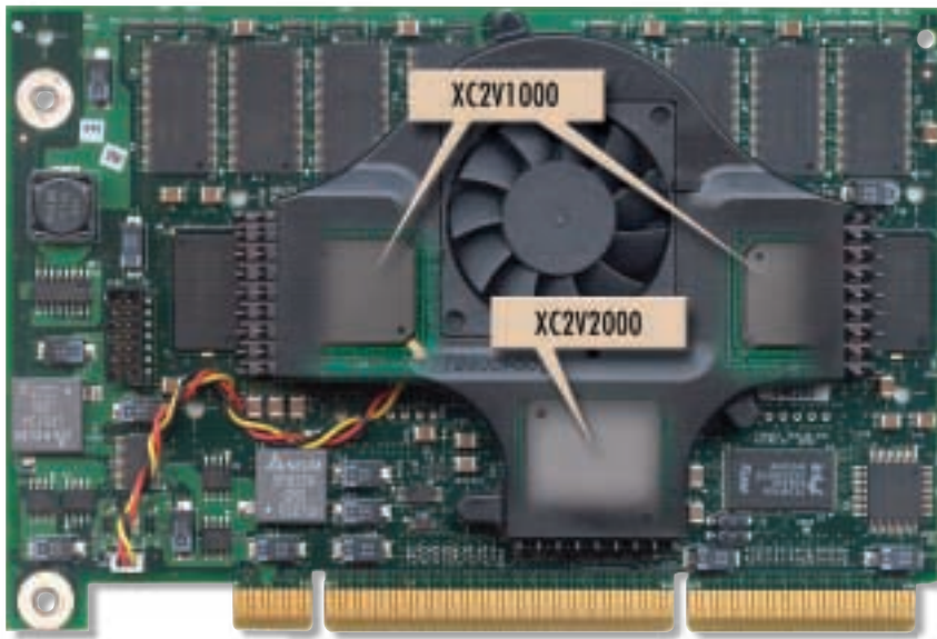
Figure 2 - Tarari PCI card with three Xilinx Virtex-II FPGAs located underneath heat sink/fan shroud
