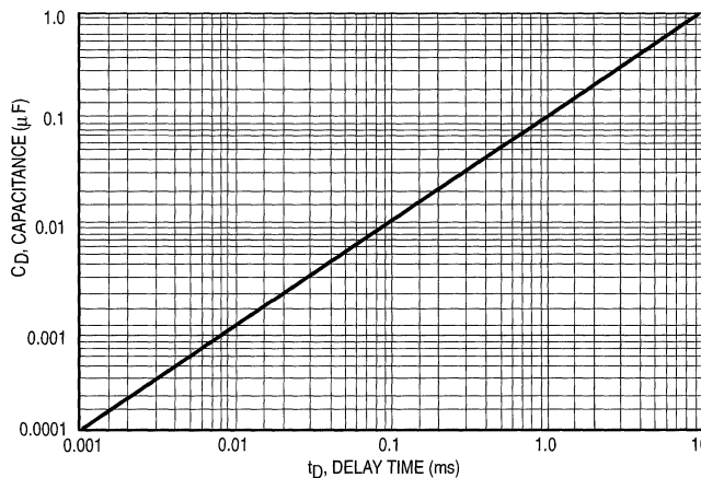
Figure 14-11. C D versus Minimum Overvoltage Duration, t D for The MC3423 OVP
