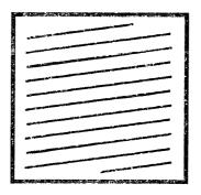
Figure 6.3: Sketch of target used for camera calibration. Lines are accurately spaced  $\frac{1}{4}$  inch (6.35 mm) apart.
