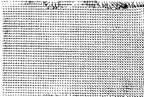
Figure 1-2: The optical flow map for the given real image sequence. The arrows show the magnitude and direction of the apparent motion at each point.
