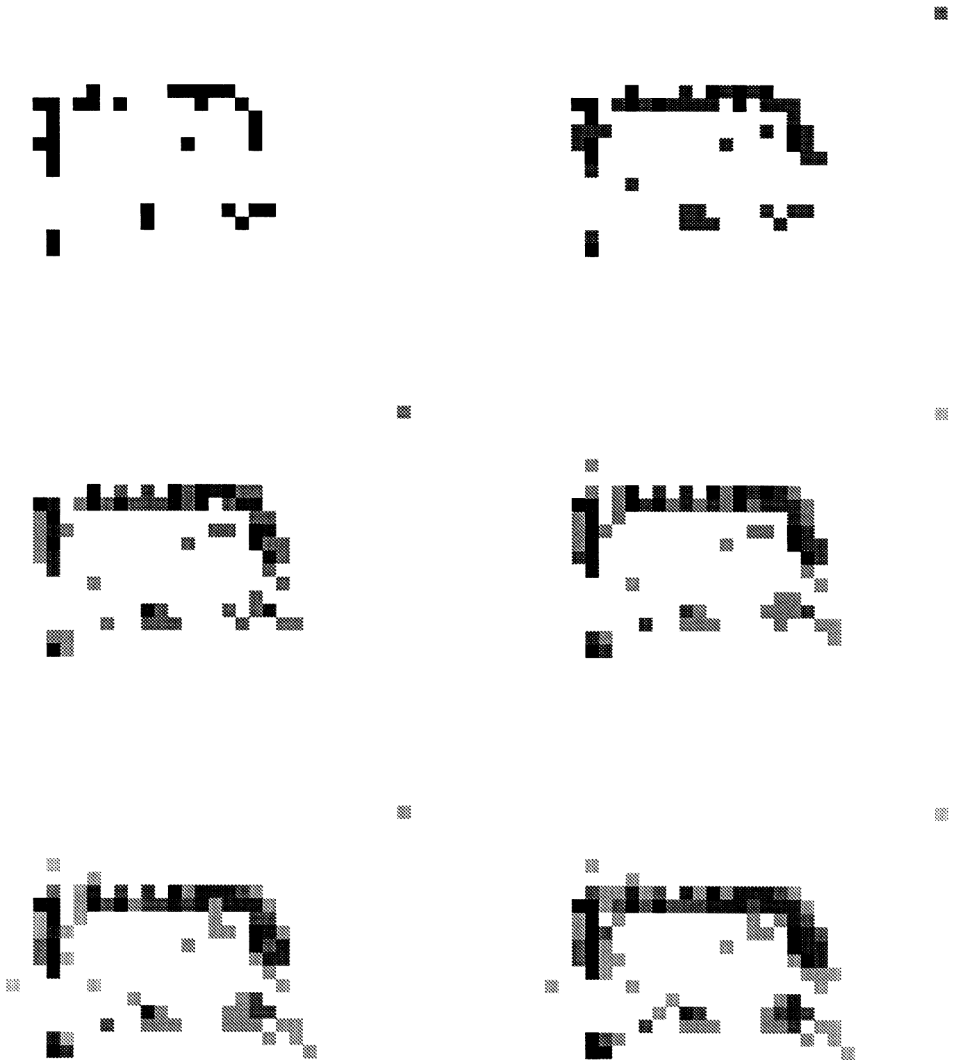
Figure 11. The weighted model for Room 914 as it evolves over the course of several recognitions. The darker squares correspond to more heavily weighted model points.
