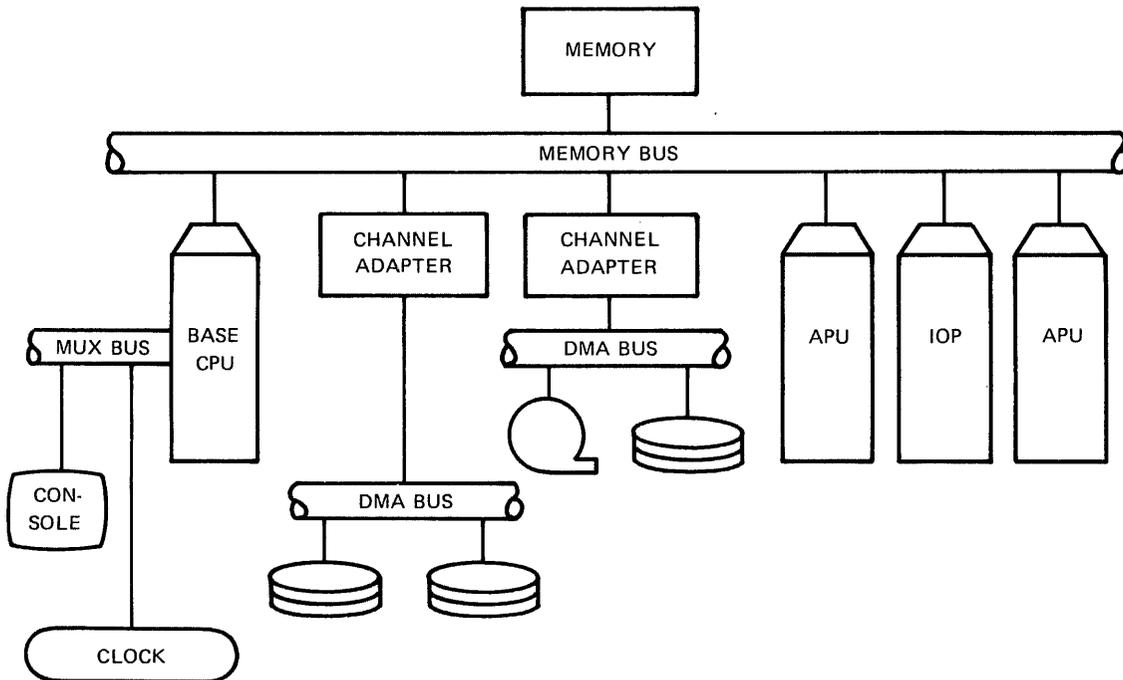
Figure 1-2 Configuration of a Typical Multiprocessing System
