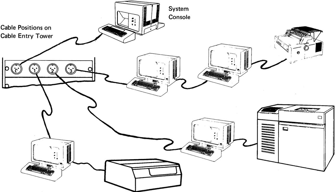
Figure 11-4. Work Station Configurations
