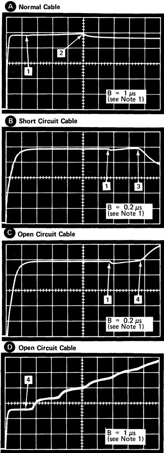
**1** A small change in the signal level caused from a terminal (with the Cable Thru feature) 131 meters (430 feet) from the end of the cable being checked. The change at **1** is also shown in **B** and **C**.
