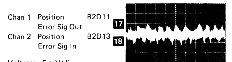
Chan 1 Position Error Sig Out B2D11 17 Chan 2 Position Error Sig In B2D13 18 Voltage: 5 mV/div Time: 2 \mu s/div Trigger: Internal + Chan 1 Vertical Mode: Add, Invert + Chan 2 Signal is inverted and therefore differential.
