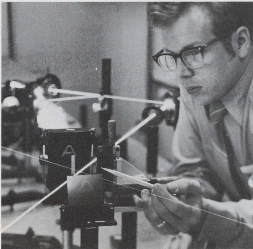
Almost simultaneous exposure and readout of holographic images occurs with a technique that does not require chemical development. Here, Scott A. Keneman of RCA watches the image of a letter as it is projected from an arsenic trisulfide thin film that is exposed to an argon laser.
