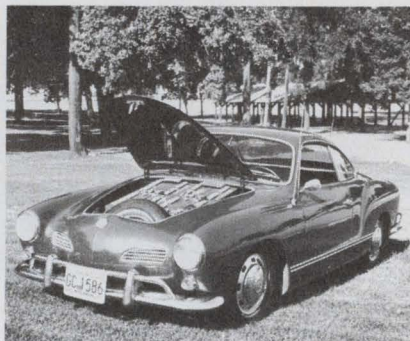
This electric commuter car developed by Allis-Chalmers Corp. uses a standard clutch and transmission.
