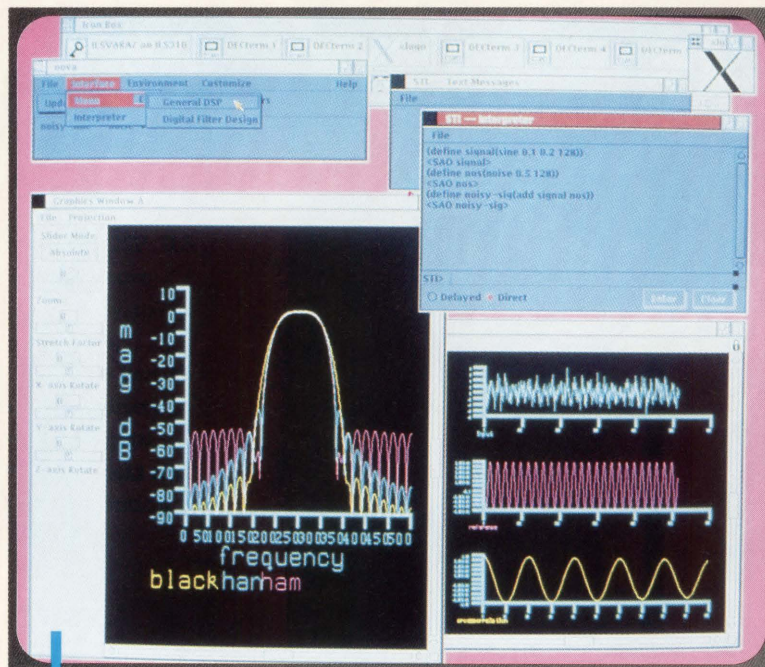
An X Window System interface display showing windowing capabilities, menu selections and graphics from N!Power.
