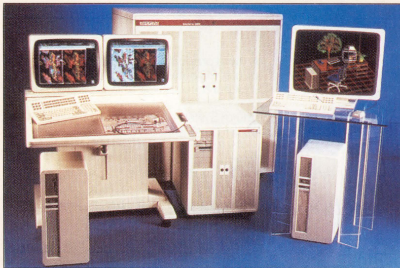
The InterPro and dual-screen InterAct 6000 Series provide more than 100 configurations at performance levels up to 14 mips.
