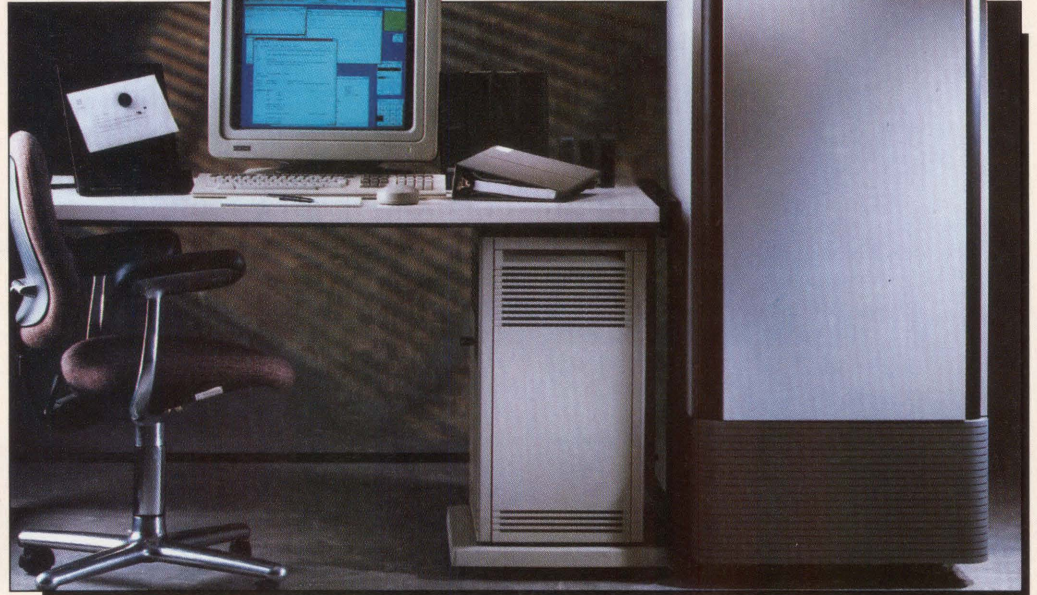
The MP 1200 Series provides up to 30,000 mips and 1,500 Mflops.
