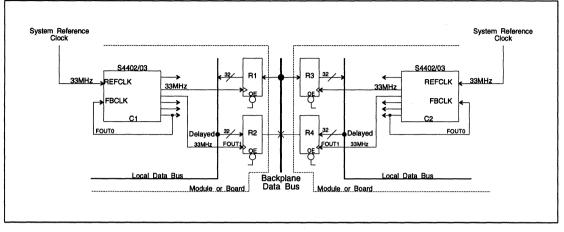
Figure 6 - Data Distribution Between Boards
