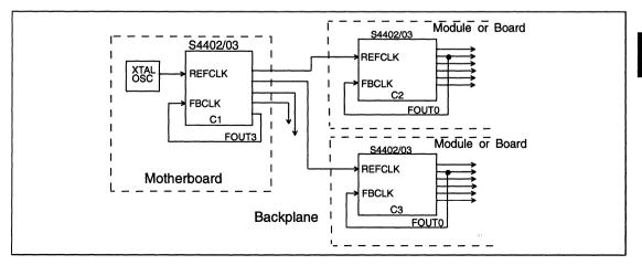
Figure 4 - Clock Distribution Between Boards
