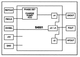
Figure 1. S4501 Block Diagram
