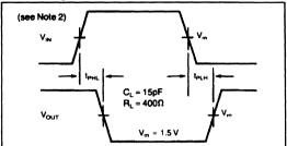
Figure 8. 2-State Waveform for Non-Inverting Functions
