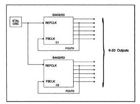
Figure 2 - Clock Distribution on a Board
