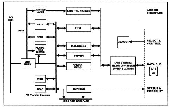
Figure 2. S5930–S5933 Block Diagram
