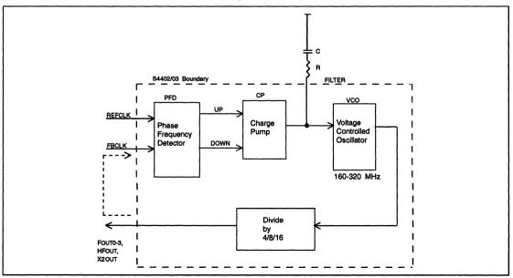
Figure 1 - Phase-Locked Loop of S4402/03
