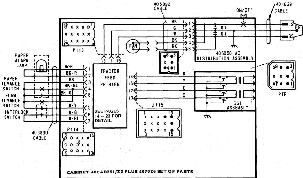
ALSO APPLIES TO 40CAB353/ZZ PLUS 405671 SET OF PARTS (TRACTOR FEED)
