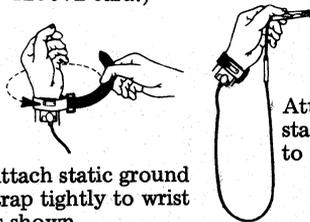
Attach static ground strap tightly to wrist as shown.
