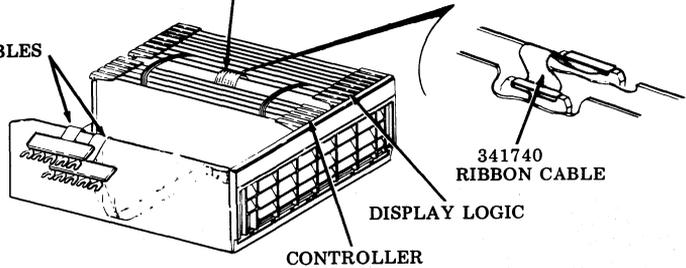
⑤ Remove controller wired frame. (Frame may still have cards mounted.)
