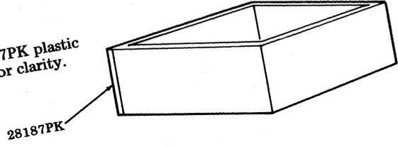
Coil cable and place between side of 28187PK detail and carton wall.
