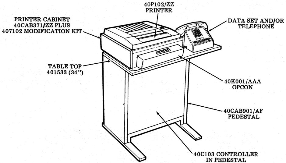
Fig. 15—40P102 Friction Feed Printer (Noise Reduced)
