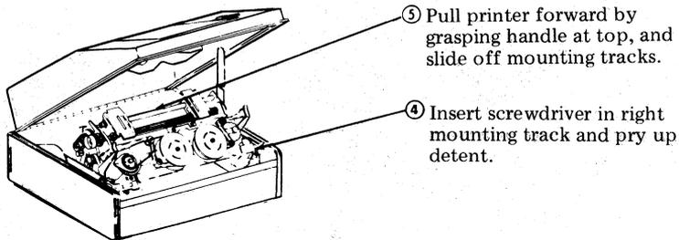
In reassembly, make sure connectors at rear are fully connected.
