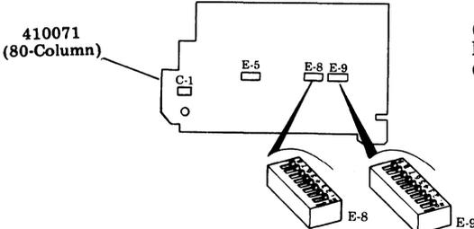
(Printer Circuit Card Viewed From Beneath Printer — Access to Switches is Through a Cutout in Bottom Pan of Printer.)
