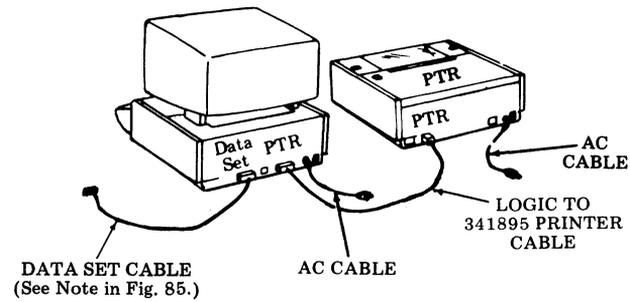
Fig. 92—KDP Table-Mounted, Adjacent Friction Feed Printer
