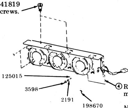
④ Remove fan assembly mounting hardware.
