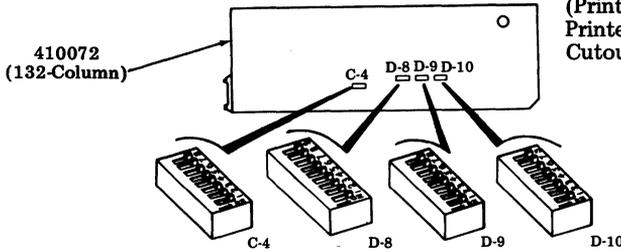
(Printer Circuit Card Viewed From Beneath Printer — Access to Switches is Through a Cutout in Bottom Pan of Printer.)
