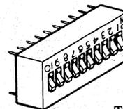
TOGGLE-TYPE SWITCH (Flip to operate.)
