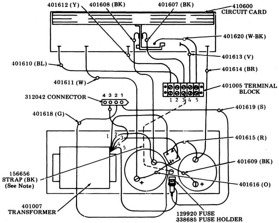
Fig. 6-40PSU101 Power Supply (Early Design)
