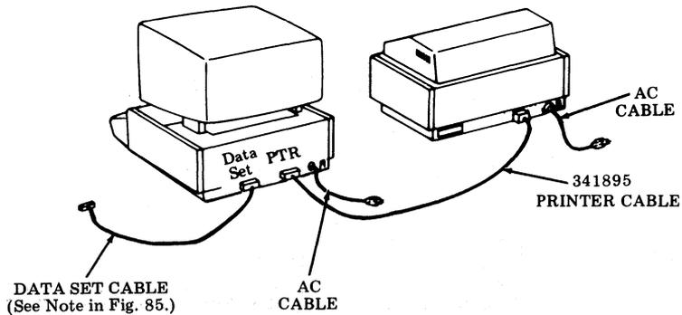
Fig. 93—KDP Table-Mounted, Adjacent Tractor Feed Printer (80-Column or 132-Column)
