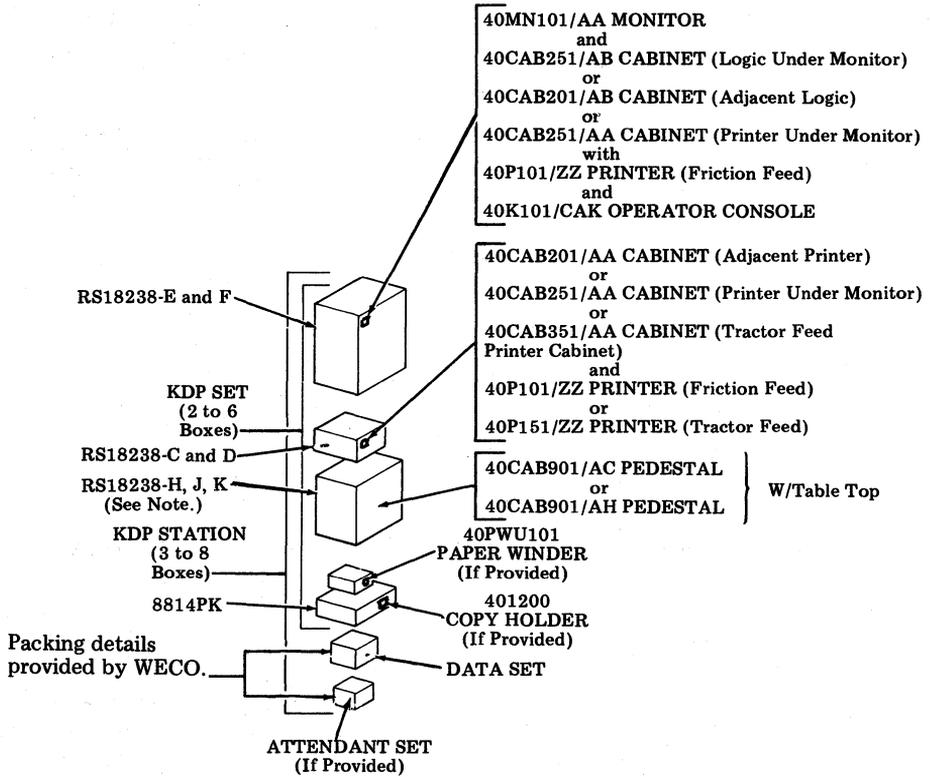
*Note:* In a KDP w/tractor feed printer on pedestal, two 40CAB901/AH pedestals must be packed.
