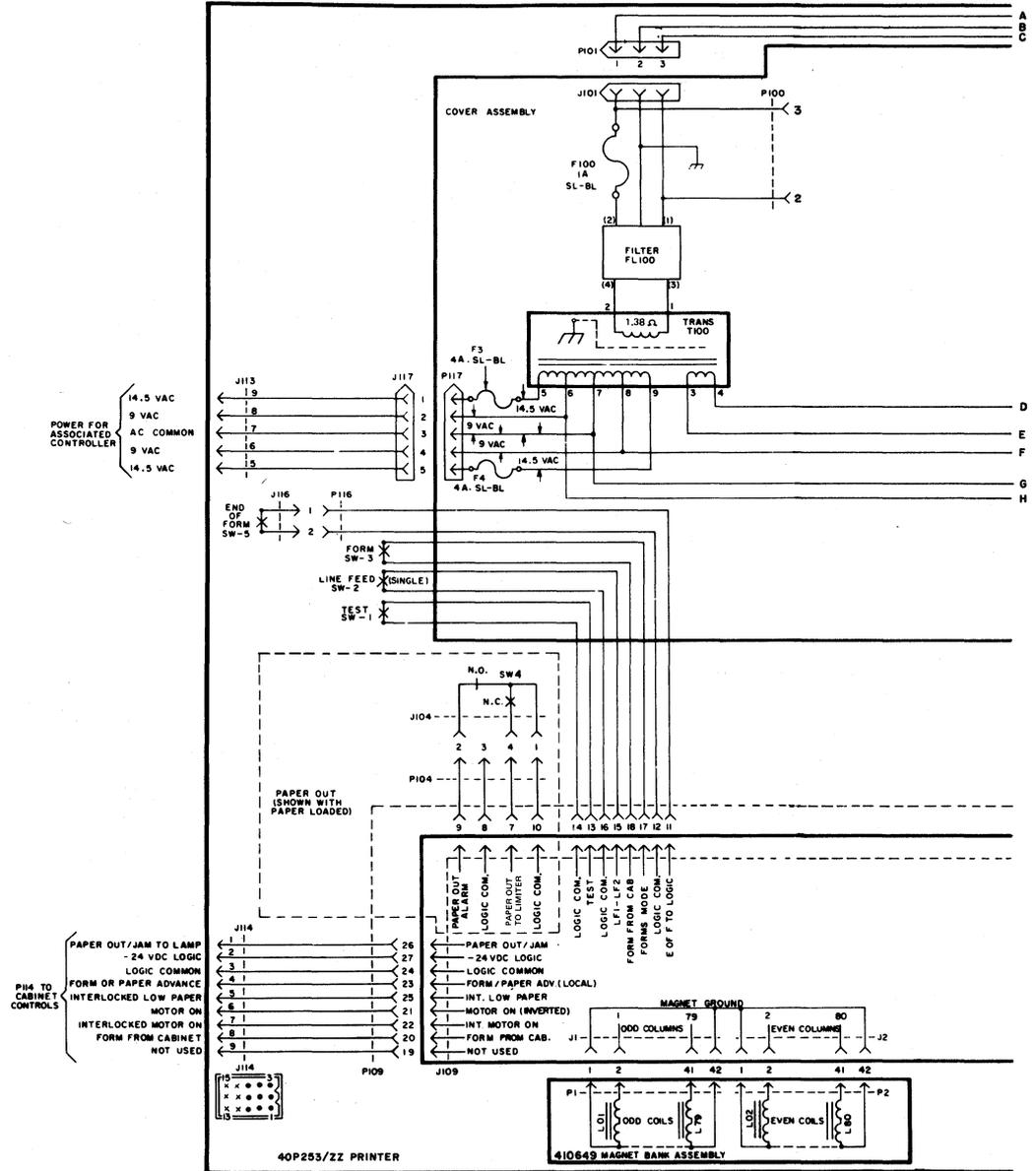
Fig. 15—40P253 Forms Access Tractor Feed Printer
