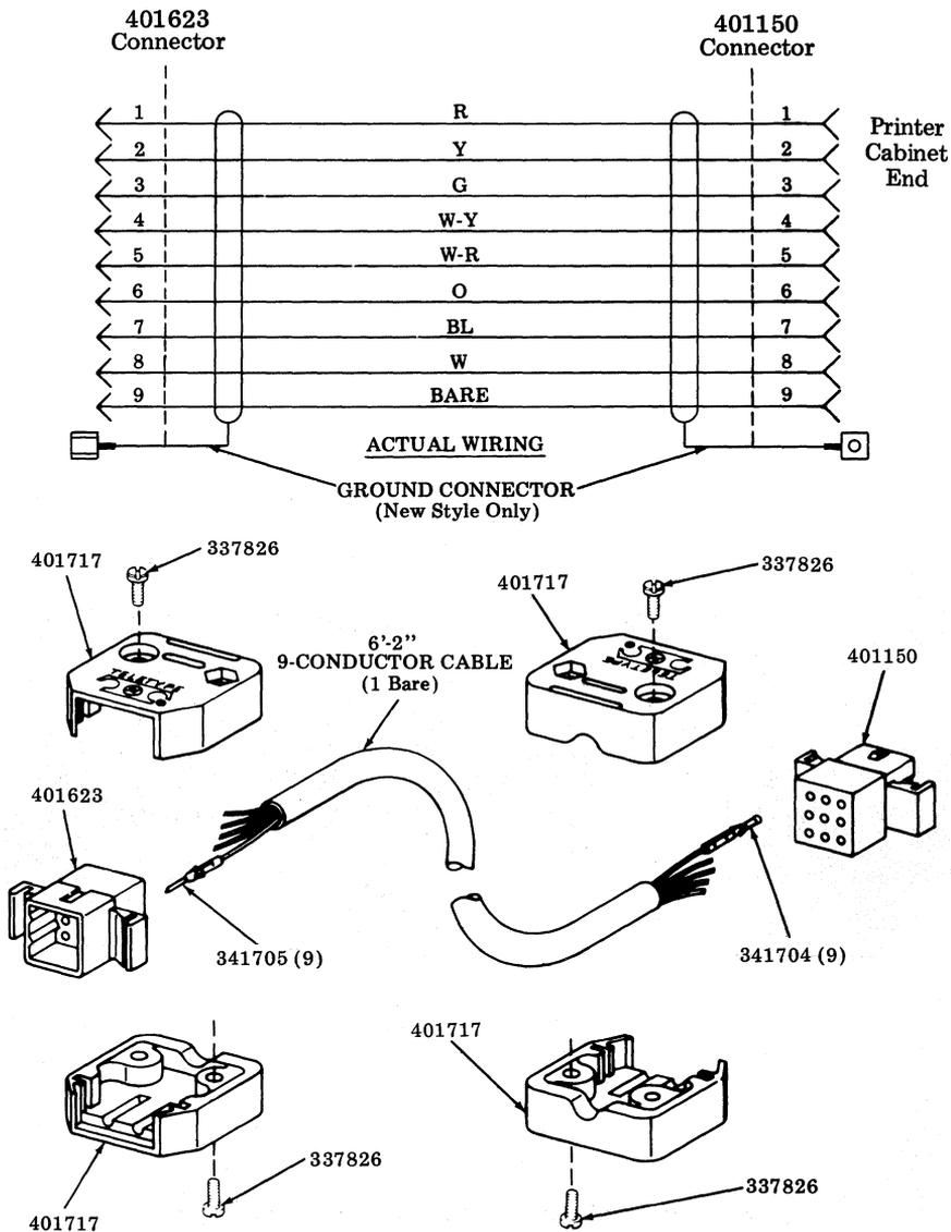
Fig. 21—401641 Opcon Extension Cable Assembly
