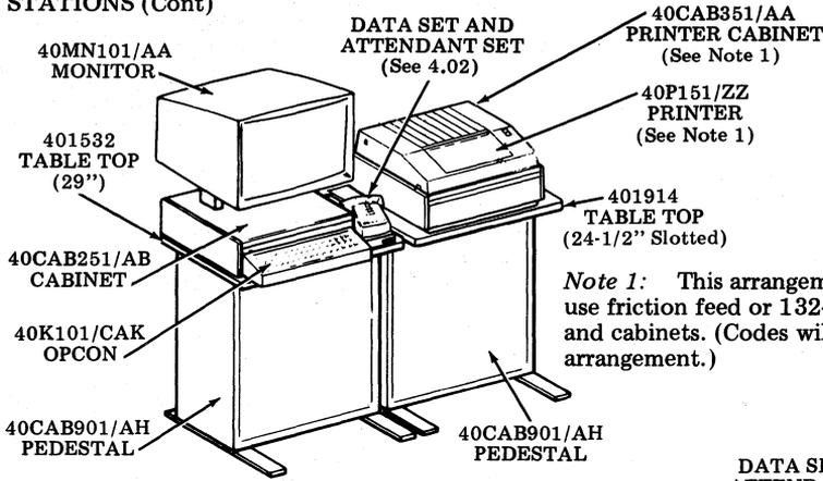
Note 1: This arrangement may also use friction feed or 132-column printer and cabinets. (Codes will vary for each arrangement.)
