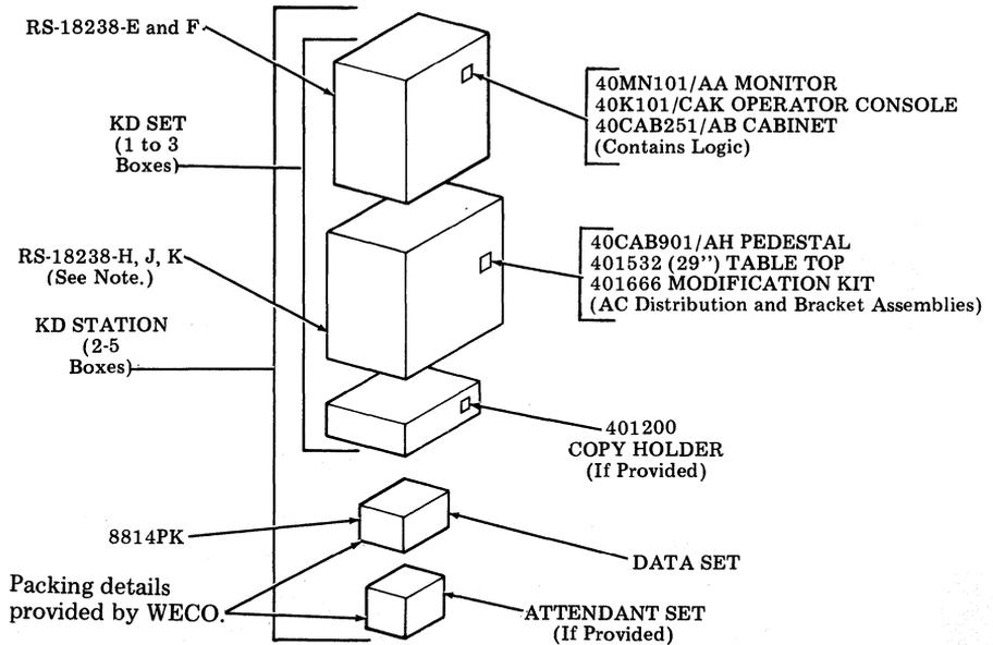
Fig. 2—Typical Packing Details for DATASPEED 40 Station Arrangements
