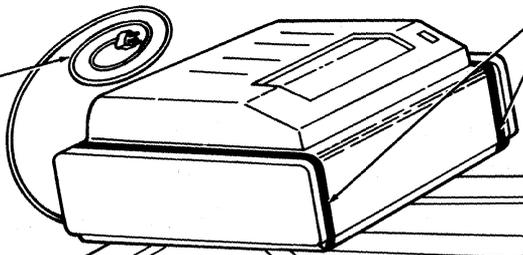
Secure cover with 2 bands of 21632PK tape applied around cabinet, as shown.
