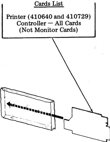
**Warning 3:** Place listed card in an RM150592 static bag immediately after removal from unit. Do not place any printer paper in the bag with the card. Keep the card in the static bag at all times. Never handle the card outside the bag without wearing a properly grounded 346392 static ground strap.
