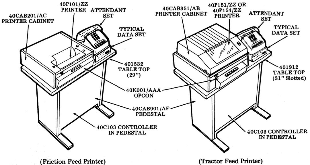
Fig. 16—ROP Station Equipped With 40C103/AD or /AE Controller
