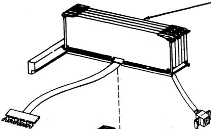
*Note:* If attendant selectable features 403400 modification kit is used, disconnect cables from 410679 circuit card.
