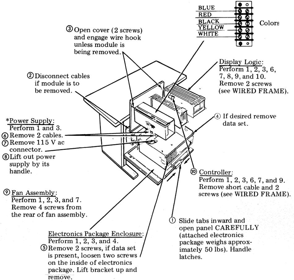
\*To reinstall power supply, seat it on locating pins in the base of the enclosure. Cables are routed over handle.
