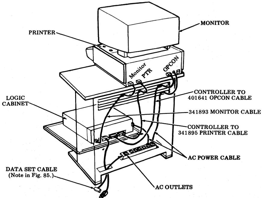
Fig. 87—KDP Pedestal-Mounted, Friction Feed Printer Under Monitor
