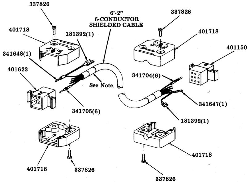
Fig. 22—401640 Printer Extension Cable Assembly (EIA)
