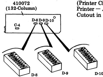
(Printer Circuit Card Viewed From Beneath Printer — Access to Switches is Through a Cutout in Bottom Pan of Printer.)
