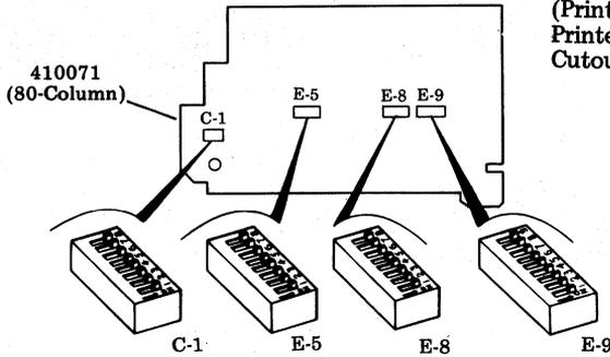
(Printer Circuit Card Viewed From Beneath Printer — Access to Switches is Through a Cutout in Bottom Pan of Printer.)
