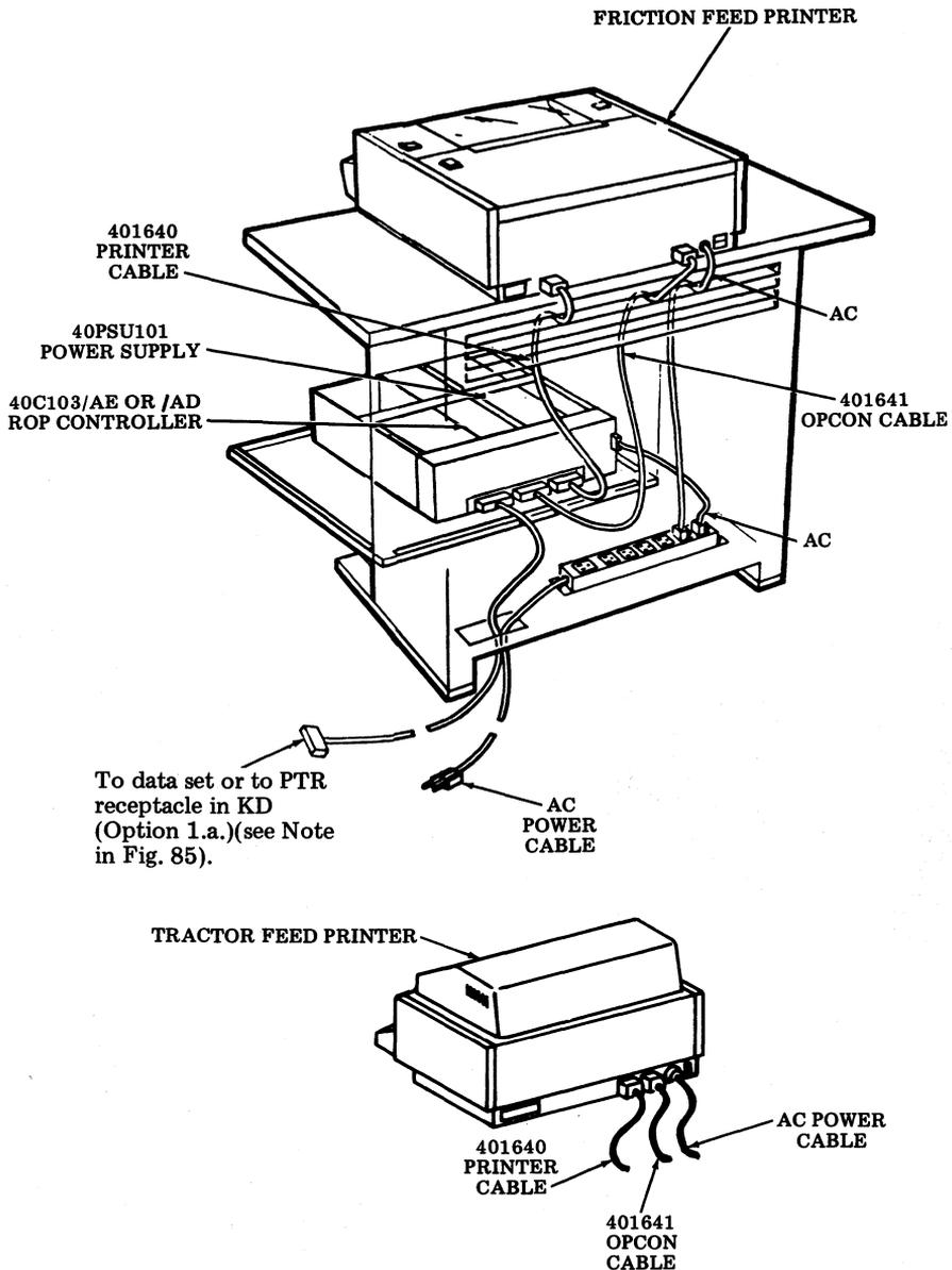
*Note:* Connection of cables is the same with tractor feed or friction feed printer.
