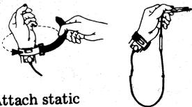
Attach clip end of static discharge strap to frame ground.
