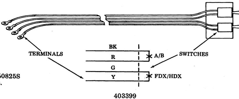
The switches mount to pedestal door, see Section 582-200-202. Terminals mount to 410680.
