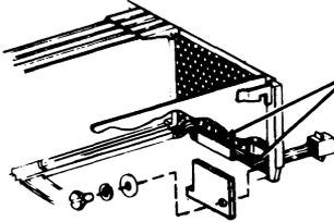
③ Remove 402166 cable protector (if present). Feed 341860 opcon cable carefully out of cable tray.
